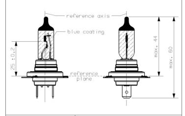
Light center length: 25mm ± 0,2mm Bulb diameter: max. 12,5mm
